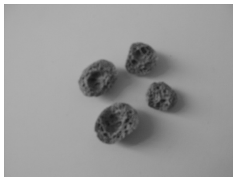
Fig.3. The macrostructure of expanded pellet (sample cross section)
